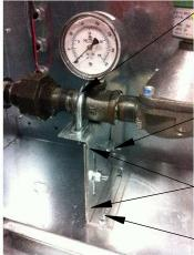
42026 3/8 U-Bolt, washer, and locknuts (2 Places)
