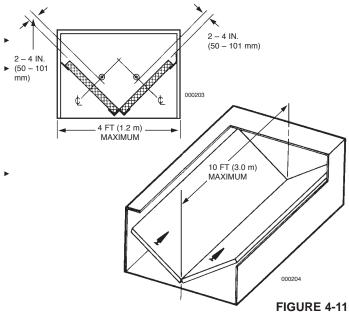
For a plenum, either single or "V" bank, with a linear extension ► longer than 10 ft (3.0 m), each bank may be protected using one
