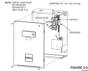
\* Note: AUTOMAN Regulated Electrical Release (Part No. 429856) is not intended to be used with electric detection. SECTION 3 – SYSTEM COMPONENTS UL EX3470 ULC EX3470
