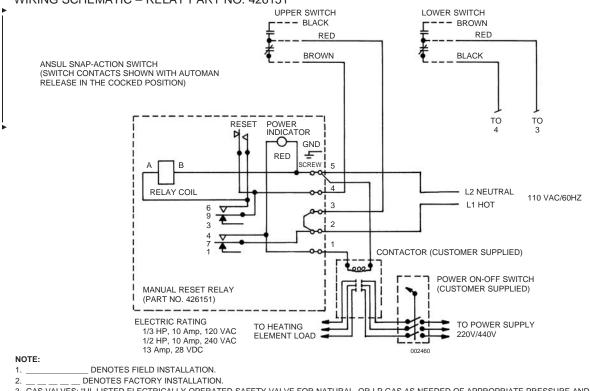
GAS VALVES: "UL LISTED ELECTRICALLY-OPERATED SAFETY VALVE FOR NATURAL, OR LP GAS AS NEEDED OF APPROPRIATE PRESSURE AND TEMPERATURE RATING, 110V/60 HZ" OR ANSUL GAS VALVES, PART NUMBERS 13707, 13708, 13709, 13710, AND 17643.
