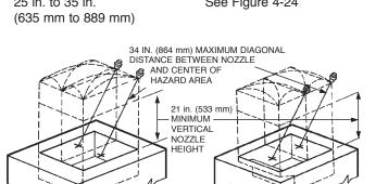
FRYER WITHOUT DRIPBOARD FRYER WITH DRIPBOARD 3N NOZZLE TIP MUST BE POSITIONED ANYWHERE ALONG OR WITHIN THE PERIMETER OF THE MODULAR IT IS PROTECTING AND AIMED AT THE MIDPOINT OF THAT RESPECTIVE MODULE AREA.
