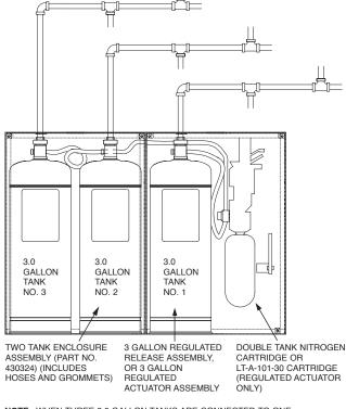
NOTE: WHEN THREE 3.0 GALLON TANKS ARE CONNECTED TO ONE AUTOMAN REGULATED RELEASE ASSEMBLY, NO ADDITIONAL REGULATED ACTUATOR(S) ASSEMBLIES CAN BE USED.
