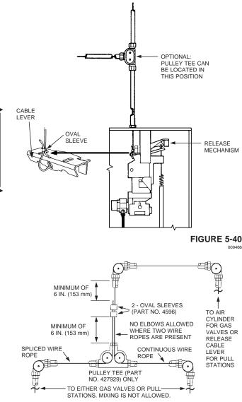
TWO WIRE ROPES CONNECTED BETWEEN A PULLEY ELBOW AND A PULLEY TEE
