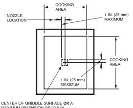
MAXIMUM DIMENSION OF 20.6 IN. (523 mm) FROM NOZZLE CENTERLINE TO FURTHEST CORNER OF GRIDDLE
