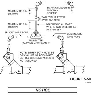
When connecting two mechanical gas valves to one air cylinder, make certain both gas valves properly operate (close) when the air cylinder rod is in the down (operated) position.
