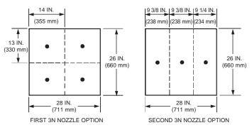
FIGURE 9-1 002466 **Example No. 2 – Fryer With Dripboard.** This fryer has an overall fry vat, including a dripboard, that measures 24 in. (609 mm) in depth x 20 in. (508 mm) in length. The actual frypot measures 20 in. x 20 in. (508 mm x 508 mm). Because both the frypot and the overall fry vat including the dripboard exceed the maximum dimensions for one nozzle, multiple nozzles will be required.
