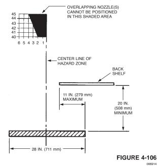
4. The overlapping appliance nozzles must be located 0 in. to 6 in. (0 mm to 152 mm) forward of the centerline or aimline of the selected hazard zone. See Figure 4-107.
