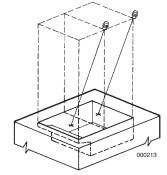
FRYER WITHOUT DRIPBOARD FRYER WITH DRIPBOARD POSITION NOZZLE TIP ANYWHERE ALONG OR WITHIN THE PERIMETER OF THE MODULE IT IS PROTECTING AND AIM AT THE MIDPOINT OF THAT MODULAR AREA.
