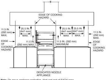
Note: On group appliance protection, start and end of EACH zone group must be protected with a 245 nozzle.
