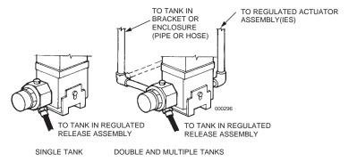
NOTE: WHEN PIPE IS USED, ALL PIPE AND FITTINGS SHALL BE SCHEDULE 40 (STANDARD WEIGHT) BLACK IRON, HOT-TIPPED GALVANIZED, CHROME-PLATED, OR STAINLESS STEEL.
