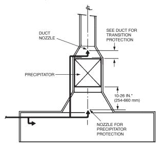
\* IF PHYSICALLY IMPOSSIBLE AT 10 TO 26 IN. (254 TO 660 mm), NOZZLE MAY BE MOUNTED CLOSER THAN 10 IN. (254 mm).
