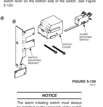
be installed on the upper tab of the switch mounting bracket.
