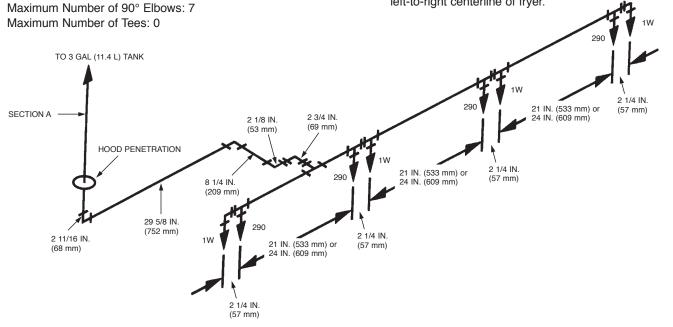
SPECIFIC DISCHARGE PIPING FOR LOW PROXIMITY PROTECTION OF FOUR DEAN INDUSTRIES MODEL GTI GAS FRYERS
