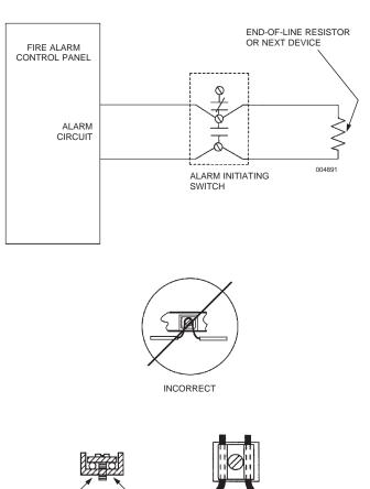
IN CORRECT - SEPARATE INCOMING AND OUTGOING CONDUCTORS
