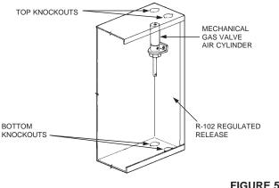
Note: Two air cylinders are necessary only if the old style pulley tee (Part No. 15342) is utilized. If new style pulley tee (Part No. 427929) is utilized, only one air cylinder is required. Individual wire ropes can be run from each gas valve to a single air cylinder. See Figure 5-45.
