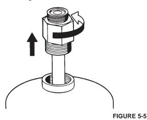
STAINLESS STEEL TANKS 2 1/4 IN. ± 1/8 IN. (57 mm ± 3 mm) FROM THE TOP OF THE COLLAR FOR THE 3.0 GALLON TANK OR 1 3/4 IN. ± 1/8 IN. (45 mm ± 3 mm) FROM THE TOP OF THE COLLAR FOR THE 1.5 GALLON TANK
