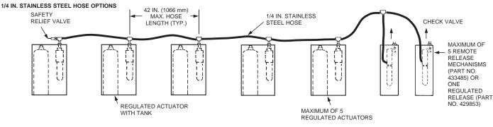
NOTE: WHEN MULTIPLE RELEASE ASSEMBLIES ARE UTILIZED, A 1/4 IN. CHECK VALVE (PART NO. 25627) WILL BE REQUIRED AFTER EACH REGULATED RELEASE.
