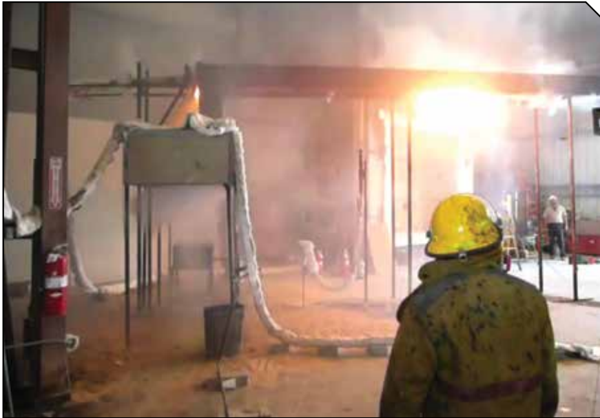
FIGURE 3. “Fireball” exploding from leaking duct during UL 300 testing.
