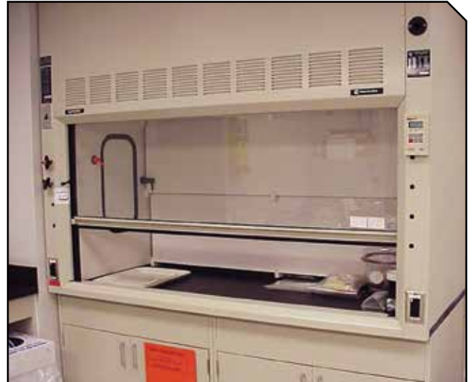
FIGURE 4. Fume hood with the equivalent of full end panels.
