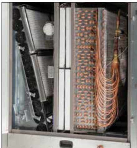
FIGURE 3. Air intake and conditioning system of a premium DOAS.
