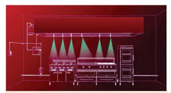
FIGURE 3: Appliance-specific pipe and nozzle design.
