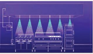
FIGURE 4: Overlapping pipe and nozzle design.
