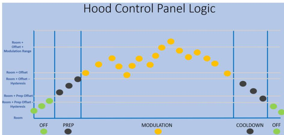
As highlighted in the graphic, the automatic operation of DCV has 3 different states.
